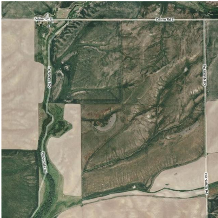
Figure 4: Zone 1 - A pattern of drainage channels that have been created the surface runoff in the area of eastern Washington where the annual runoff is between 1-5 inches/yr. (aerial photograph is downloaded from Bing Maps).
